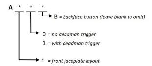
Example: A31B = A-style handle, 3 buttons on the front faceplate, deadman trigger, & optional backface button
